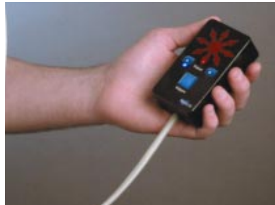
The hand worn Package Compass, which is connected to the server. The cable in this case shall be replaced by a wireless link.
