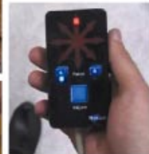
The handheld unit shows the way to the selected package with LEDs
