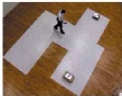
The packages placement is registered by RF-tags under the carpet
